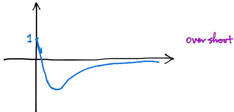
$$\begin{aligned} \alpha &< -5 \\ y(t) &= (1 + (\alpha + 5)t) e^{-5t} \end{aligned}$$
